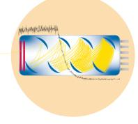
Quantitative low-light measurement Cooled PMT reduces background noise allowing for a more sensitive, wide dynamic range in extremely low light.
